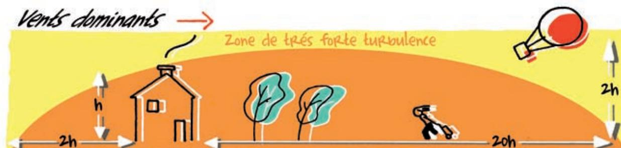
LES VITESSES DE VENT DIMINUENT ET LES TURBULENCES AUGMENTENT EN AVANT D'UN OBSTACLE... MAIS AUSSI EN AMONT.
